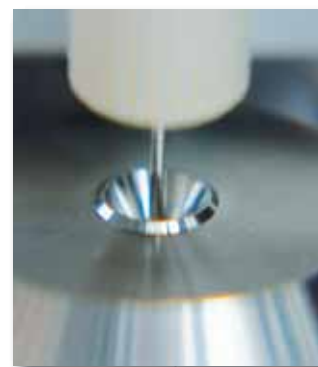
◀ Direct injection: Acidifying, purging, injecting
